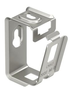
Metal grouped support for high mechanical stability, even in case of fire. Suitable for secure mounting above fire protection ceilings. Also approved as a cable-specific variant for the maintenance of electrical function to DIN 4102 Part 12. For wall and ceiling mounting. Lock can be opened without tools. Detailed information on the approved routing variants can be found in the appropriate testing documentation.
