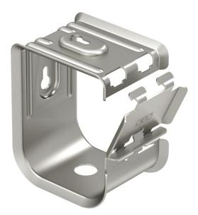
Metal grouped support for high mechanical stability, even in case of fire. Suitable for safe mounting above fire protection ceilings. Also approved as a cable-specific variant for the maintenance of electrical function to DIN 4102 Part 12. For wall and ceiling mounting. Lock can be opened without tools. Detailed information on the approved routing variants can be found in the appropriate testing documentation.
