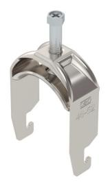
Clamp clip with U-foot, metal pressure sleeve with rounded edges to protect the cable. For vertical and horizontal mounting of 1 single cable on a C-profile rail. For slot width 18–22 mm. With 1-start screw thread on pressure sleeve, universal hexagonal screw head WAF10, with slot and cross recess. Suitable for assembly indoors and outdoors. We recommend the use of a counter-sleeve.
