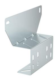
Mounting plate for the fastening of junction boxes of the FireBox T series (with external fastening) onto cable trays or cable ladders with a side height of 60 mm. The angled construction from sheet steel reinforced through crimps enables the secure mounting of cables that maintain electrical functionality, without having to bend the cable over the side rail.
