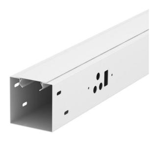
Supermarket trunking system for suspended mounting. The system is used for cable routing and device installation. Trunking length with perforations for device installation. The prepunched trunking contains the following perforations for every 3 m in length: 6x Crabtree 16A SSO, 4x insulator, 4x 32A and 5x Pin Panel socket.
