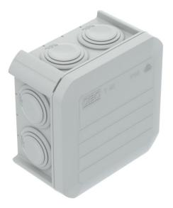
Junction box for the connection of cables indoors and in protected outdoor areas. Square design with plug-in seals to the sides and knock-out entries in the bottom. Suitable for wall and ceiling mounting and on mounting panels. With the option to fasten inside. With fixed clamping cover. Made from halogen-free, UV-resi-
