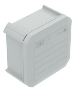
Junction box for the connection of cables and lines indoors and in protected outdoor areas. Square design without entries. Suitable for wall and ceiling mounting and on mounting panels. With the option to fasten inside and to mount via the corner domes. With fixed clamping cover. Made from halogen-free and UV-resistant materials.
